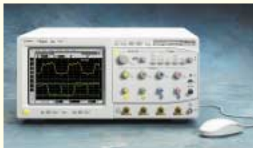
1. The 4-GHz model 54854A and 6-GHz model 54855A Infinium digital oscilloscopes provide sampling rates to 20 GSamples/s simultaneously on four independent channels.
